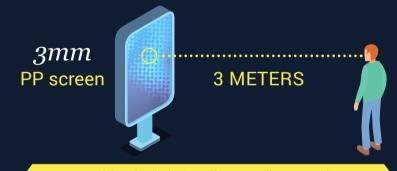
Thus, at a viewing distance of 3 meters (9.8 feet), the optimal pixel pitch would be 1.2mm, and the acceptable pixel pitch would be 3mm.
