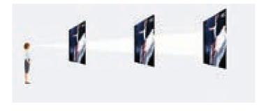
Pixel pitch is the distance from the center of a pixel to the center of any adjacent one. The smaller the pixel pitch, the higher the density and the clearer the image. Greater pixel density carries a higher price tag, so the best way to choose the right option is to consider the optimal viewing distance for the type of content - whether its text, images or video; and its application - whether for company presentations or for digital signage.
