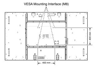
Mounting accessories can be attached with the monitor in the face down position. To avoid damaging the screen face, place the protective sheet on the table underneath the LCD. The protective sheet was wrapped around the LCD in the original packaging. Make sure there is nothing on the table that can damage the monitor. When using mounting accessories other than NEC compliant and approved, they must comply with the VESA-compatible mounting method.
