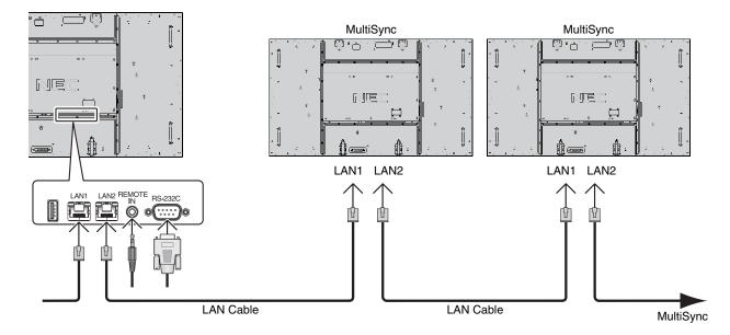
This LCD monitor can be controlled by connecting a personal computer with a RS-232C (reverse type) terminal.
