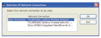
Select the network device displaying "Easy Connection" if the product LAN setting is for "Easy Connection." This will call up the "Projector List" window.
