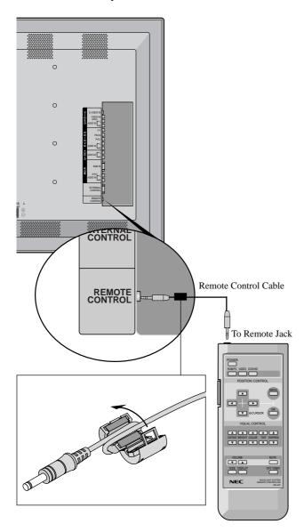
**Note:** When you connect a remote control cable to this monitor, attach the supplied ferrite core. If you do not do this, this monitor will not conform to mandatory FCC standards.
