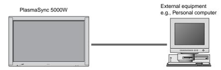
1) Connector on the PlasmaSync 5000W side: EXTERNAL CONTROL connector.
