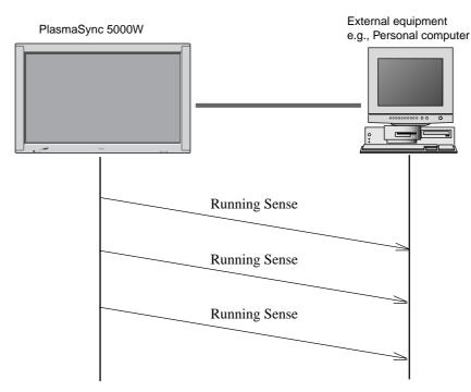
The PlasmaSync 5000W regularly transmits a Running Sense command at an interval of approximately 1 second. (Running Sense command: 1FH 60H E0H 88H 00H E7H)
