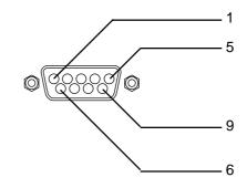
Connector on the external equipment side: Serial port (RS-232C) connector See the specifications of the equipment that is to be connected for the type of connector and the pin assignment.
