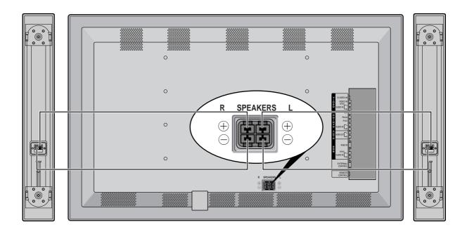
External speakers may be connected to the PlasmaSync 5000W to reproduce sound from VIDEO, DVD or RGB signal sources.
