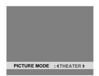
\* If neither the ◀ or ► button is pressed within 5 seconds, the current selection is set and the previous screen reappears. 4. Press the "OK" button. The picture mode is set to "THEATER".
