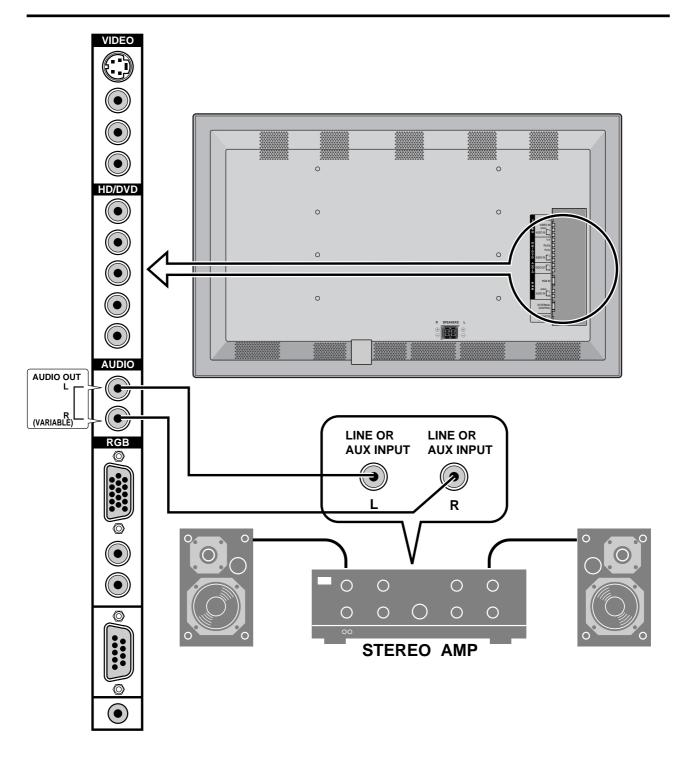
To connect the PlasmaSync 5000W to stereo system speakers:
