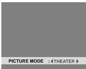
\* If neither the ◀ or ▶ button is pressed within 5 seconds, the current selection is set and the previous screen reappears.
