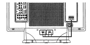
To connect the monitor to stereo system speakers:
