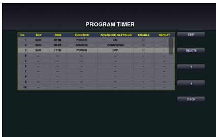
By setting day and time onto the projector, it enables the projector to automatically switch the power, the condition of standby, the video signal and the condition of ECO mode. As an example based on the above, every Sunday projector is powered on at 9 AM, is switched to the computer display at 9:03 and is gone into the Standby condition at 17:30.
