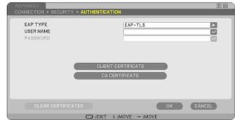
Select either [EAP-TLS] or [PEAP-MSCHAPv2] for [EAP TYPE]. The setting items vary depending on the EAP type.
