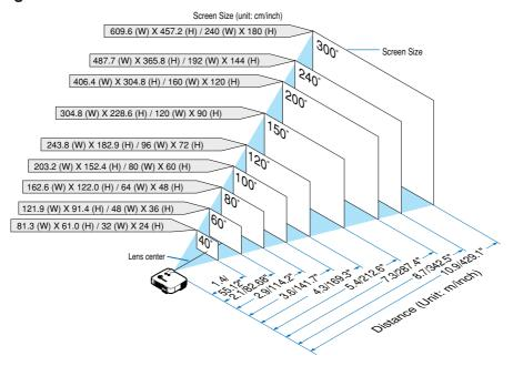
**TIP:** The screen sizes above are intermediate values between tele (minimum display area) and wide (maximum display area) when the standard lens is used. Image size can be adjusted with the zoom adjustment up to a maximum of 15%. For optional lenses, see page 113.
