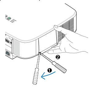
2. Loosen the two screws securing the lamp housing until the phillips screwdriver goes into a freewheeling condition. The two screws are not removable.
