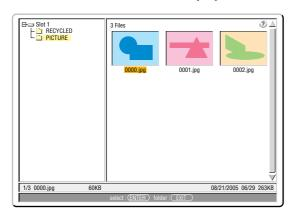
NOTE: To change highlight from the Thumbnails screen (right window) to a directory tree (left window), press the EXIT button. To return highlight to the Thumbnails screen, press the ENTER button.
