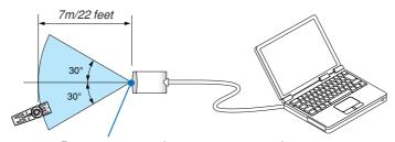
Remote sensor on the remote mouse receiver
