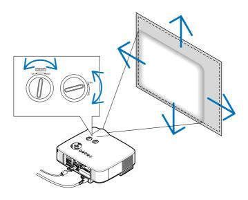
NOTE: The lens shift dial for LEFT-RIGHT cannot be rotated one-half turn or more. Do not over rotate it or it may break.
