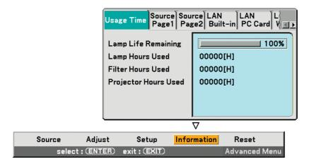
Displays the lamp and the projector usage hours, the status of the current signal and settings and LAN settings. This dialog box has seven pages.
