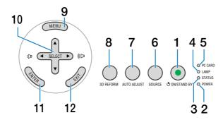
1. POWER Button (ON / STAND BY) (→ page 24, 35) NOTE: To turn on the projector, press and hold this button
