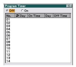
This option turns on or off the projector automatically at a specified time. Up to 14 different timer settings can be programmed.
