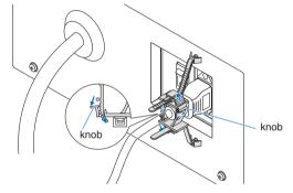
This completes the attachment of the power cable stopper.
