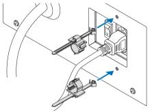
**2** Pass the band through the slits in the power cord stoppers.
