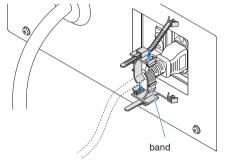
3 Slide the clamper unit to the base of the power cord.
