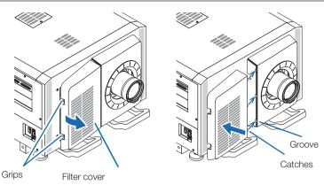
The illustration in this explanation shows how to clean the air filters on the top panel. Clean the other filters in the same way as these air filters (small type).
