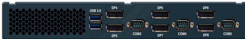
**Figure 2. NETPC-BD6C Back Plate. MXM Graphics Card Display Ports.**
