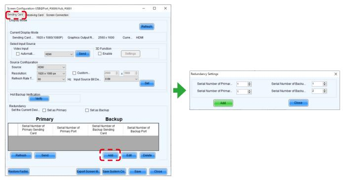
In the Redundancy Settings screen, set the Port number of the Backup side LED controller (Sending Card) that matches the Port number of the Primary side LED controller (Sending Card).
