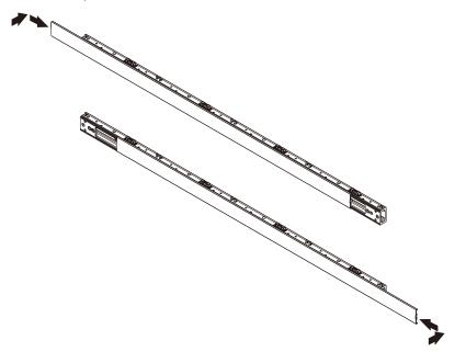
Insert the slot nut into the overframe and align it with the marking line and fix them with screw for overframe screws.
