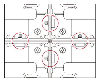
After you have installed two rows of cabinets, align the surfaces of the cabinets using the Adjustment plates.
