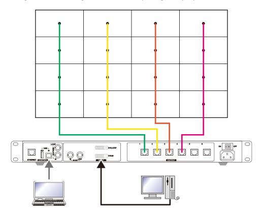
(1) With a pixel pitch of 1.25 mm, enter Width=480 and Height=270 under "Receiver Card Size" (e). Do not use the buttons located next to the values.
