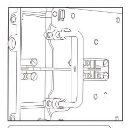
When carrying or installing the cabinet, pull out the handles on both sides.
