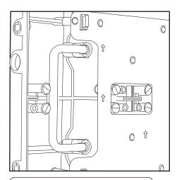
Put the handles back after the work has been completed.
