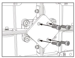
Adjust the position of the cabinet by turning the vertical alignment screw and the back in the center of the vertical alignment screw (cabinet hanger pin) with a flathead screwdriver.
