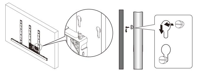
Fix temporarily the cabinets of the first row to the power bar.
