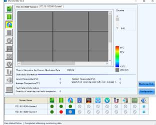
Note: On the monitoring screen, the LED modules configured as "Backup" are displayed in red color (this is not an indication of a fault).
