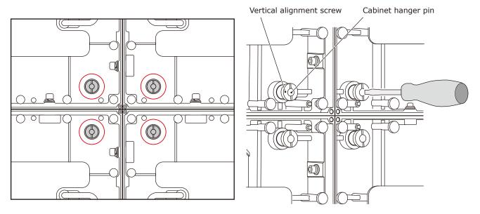
When the cabinets' surfaces are aligned, securely tighten the cabinets of the first row to the power bar, the cabinets of the first row together, as well as the cabinets of the first row with the cabinets of the second row. Remove the Adjustment plates after the screws have been tightened.
