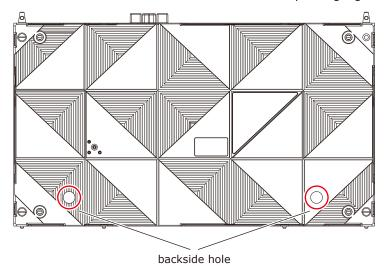
If the hole is not drilled, place a flathead screwdriver from inside the cabinet at the edge of the round recess and tap it lightly with a hammer to make a hole.
