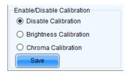
(10) If calibration-setting "Disable Calibration" is chosen, switch to "Chroma Calibration" (c) to enable calibration and click on the "Save" button (d).
