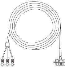
To connect the LED module to the power distributor
