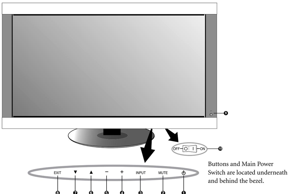
Buttons and Main Power Switch are located underneath and behind the bezel.
