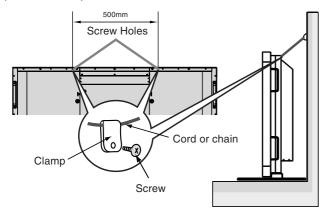
Before attaching the LCD monitor to the wall, make sure that the wall can support the weight of the monitor.
