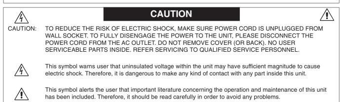
**CAUTION:** Please use the power cord provided with this display in accordance with the table below. If a power cord is not supplied with this equipment, please contact your supplier. For all other cases, please use a power cord that matches the AC voltage of the power outlet and has been approved by and complies with the safety standard of your particular country.
