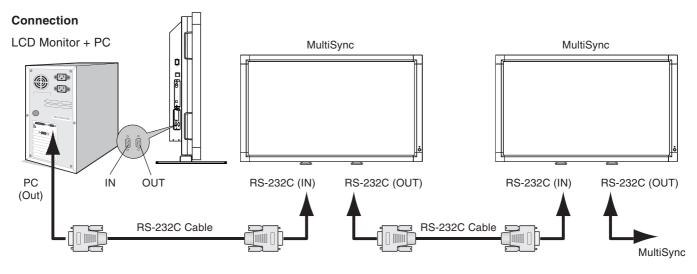
**NOTE:** If your PC (IBM or IBM compatible) is equipped only with a 25-pin serial port connector, a 25-pin serial port adapter is required. Contact your dealer for details.
