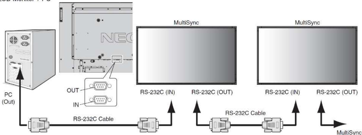
(Please refer "Controlling the LCD monitor via RS-232C Remote control" on User's manual.)
