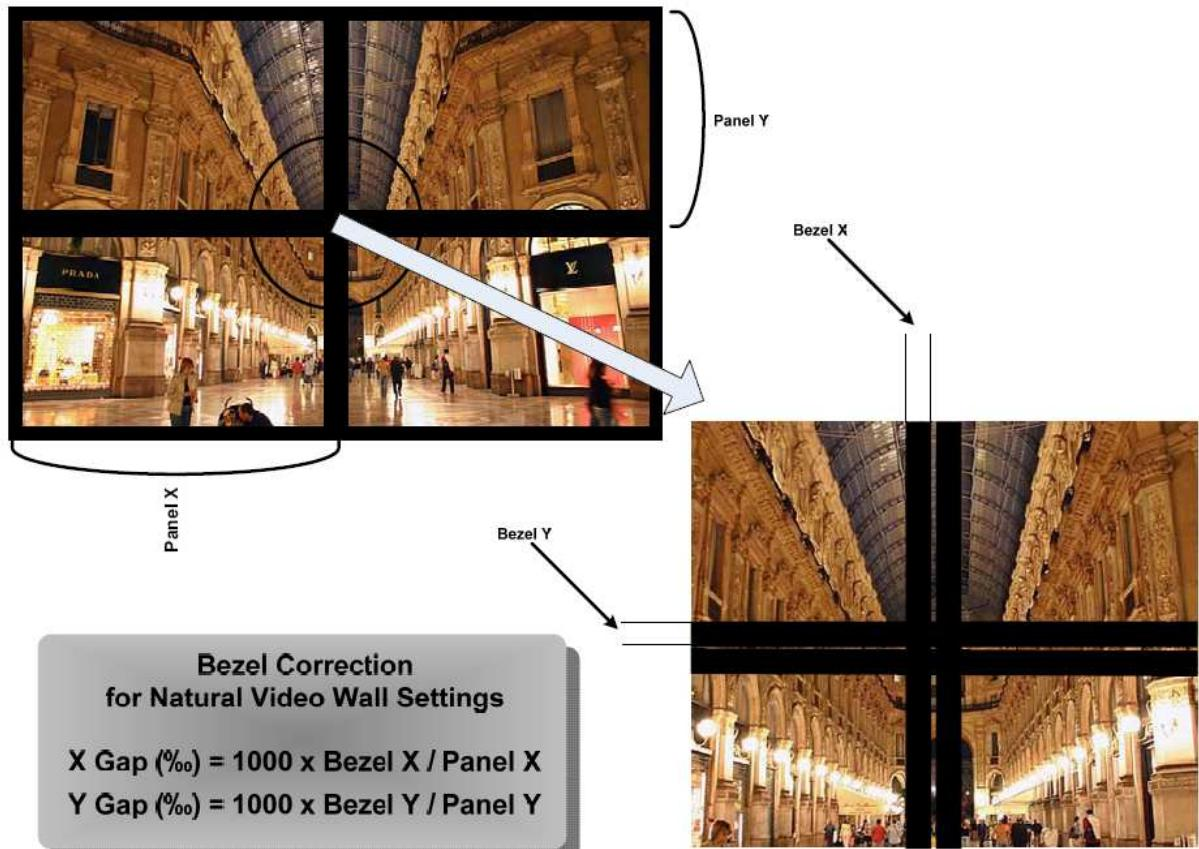
**X Gap** : Proportional Value of Vertical Bezel to Panel size by Per-mil unit.
