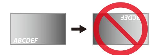
The monitor cannot be used when inclined  $15^\circ$  or more.
