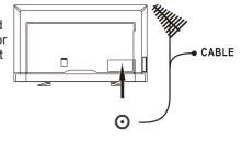
When using a 75-Ohm coaxial cable system, connect the CATV coaxial cable to the AIR/CABLE (75-Ohm) terminal. Or if you have an antenna, connect the coaxial cable to the same AIR/CABLE terminal.
