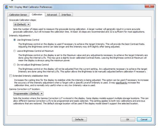
**Calibration and Profile Steps** - Selects the number of measurement steps to take when calibrating the display. A larger number of steps will generally result in a more accurate grayscale calibration, but will increase the calibration time. 16 steps is the recommended setting for most applications.
