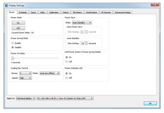
The **Power** tab controls the power settings of the displays.
