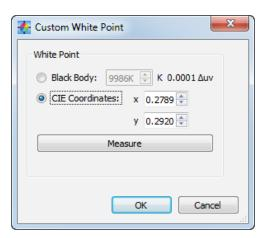
The **Custom White Point** dialog is accessed by clicking the **Edit.** button in the **White Point** section of the **Edit Calibration Target** dialog.
