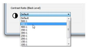
Selecting **Default** will calibrate the display to the highest possible contrast ratio, which is limited by the display technology, the selected White Point, Intensity value, and other factors.
