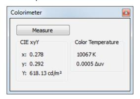
This panel allows measurements of colors displayed on the screen to be taken with the calibration sensor and the numerical results are displayed.
