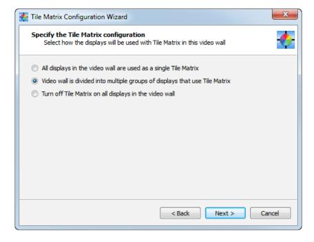
The Wizard can be used to enable a single tile matrix across all displays in the current project, or to configure multiple groups of displays within the project, or to disable Tile Matrix on all displays.
