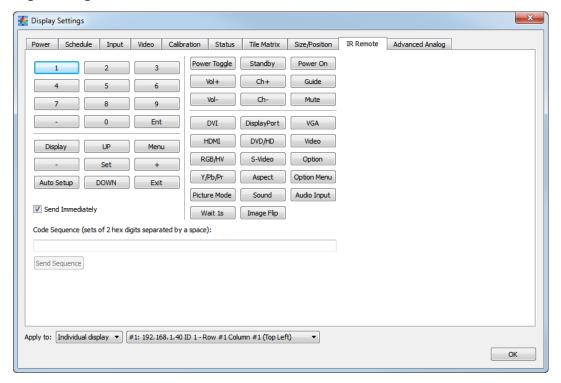
The *IR Remote* tab can be used to perform the equivalent operations as the physical IR Remote control using the software and communicating using the LAN or RS232 connection to the display.
