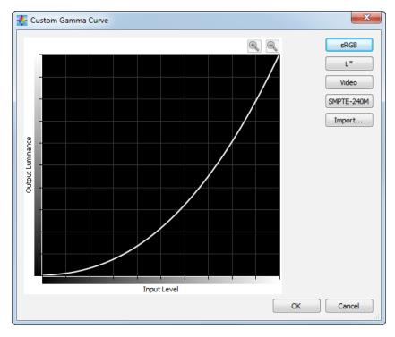
The **Custom Gamma Curve** dialog is accessed by clicking the **Edit.**. button in the **Gamma Curve** section of the **Edit Calibration Target** dialog.
