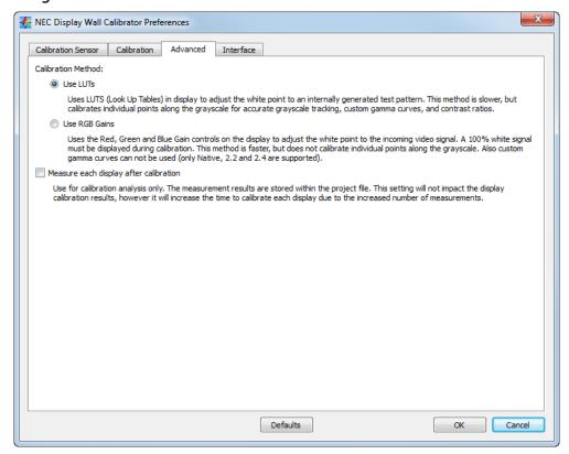
Calibration Method - Selects the how the calibration is performed in each display. Options are:
