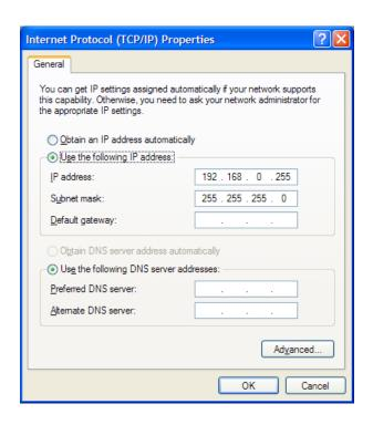
Next enter a temporary IP address for the PC, such as 192.168.0.255, and a subnet mask of 255.255.255.0. Click *OK* and close the Network Settings.
