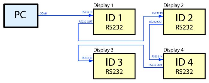
**Note:** For RS232 daisy-chains, the cable connections between displays does not need to follow the same ordering as the ID assignments. In this example the daisy-chain is connected in order 1 - 2 - 4 - 3.
