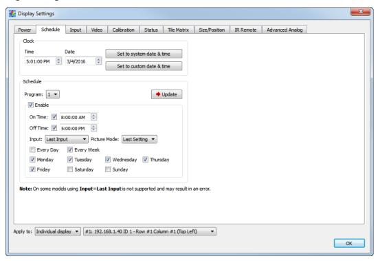
The **Schedule** tab is used to set the internal real time clock and schedule functions in the display. Various scheduled operations such as power on, power off, and changing inputs can be configured.
