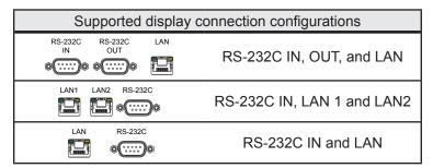
Models that have an RJ45 LAN connection can be individually connected directly to a LAN via a hub or switch instead of daisy-chaining displays together. This may require more wiring since each display is individually connected directly to a central LAN hub or switch. The advantages of using this method is that communications to other displays will still function even if:
