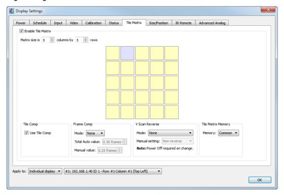
The *Tile Matrix* tab can be used to configure the Tile Matrix settings for dividing and expanding a video source over multiple displays.
