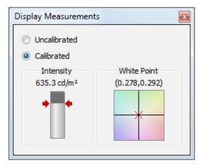
This panel shows the measured White Point values from the color sensor taken during the Measurement and Calibration operations. Both the White Point and Intensity (luminance) are shown as numerical values and graphically.
