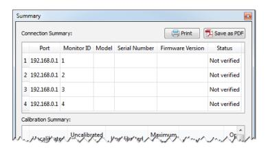
**Note:** Since the Monitor ID numbers are assigned sequentially based on the physical connection order of the displays when the Auto ID operation is performed, the layout and ID assignments in the software must match accordingly.
