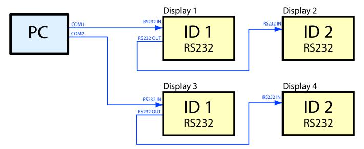
The following image shows how this layout looks in the Summary window when configured. Notice that displays connected on COM1 can have the same IDs as those on COM2 because they are on separate daisy-chains.
