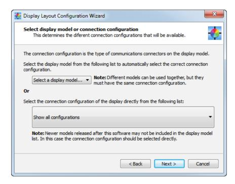
Selecting by display model will automatically select the correct connection configuration. Alternately the connection configuration can be selected from the list as shown below.
