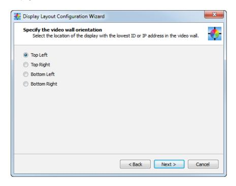
Next the order of remaining displays can be selected. This selection determines how sequential IDs or IP addresses will be automatically assigned to the rest of the displays, and the order of measurement and calibration. Keep in mind that the automatically assigned IDs or IP addresses can be modified later if necessary, as well as the measurement and calibration order.
