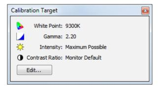
This panel shows the Calibration Target settings that will be used when the displays are calibrated.
