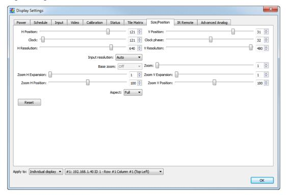
The *Size/Position* tab can be used to configure the various video size and position settings in the display. When *All Displays* is selected, controls are not updated until the associated update button is clicked.
