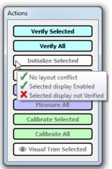
Each button has a ToolTip which shows the steps and conditions necessary for it to be enabled. Hold the cursor over a button and the ToolTip will list the conditions. A green check mark 🗸 indicates that a condition has been met. A red cross mark 🗶 indicates that a condition has not yet been satisfied. When all conditions have been satisfied the button will be enabled.
