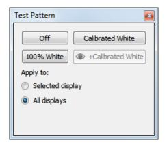
This panel is used to display test patterns on either the currently selected display, or all of the displays in the layout.
