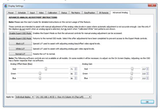
The **Advanced Analog** tab can be used set special video adjustment patterns used to assist with manual adjustment of the analog video input levels.
