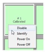
**Disable** - An individual display can be excluded from the current project by disabling it. To disable a display, right click within the rectangle and select Disable. This feature can be used for example if the video wall layout is not a rectangular shape.
