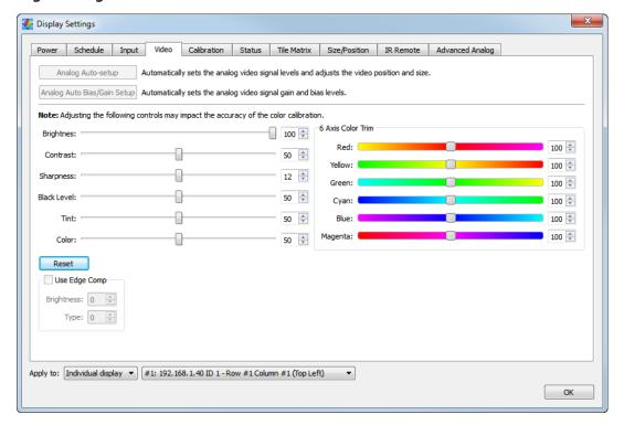
The Video tab is used to perform video signal and color adjustments.
