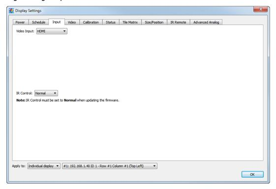
The *Input* tab is used to set and report the current video input selected on the display, and also the IR Control setting.
