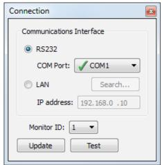
This panel is used to modify the communications connection settings for the currently selected display in the layout.
