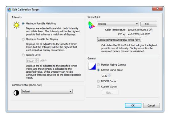
The Edit *Edit Calibration Target* dialog is accessed by clicking the *Edit...* button on the *Calibration Target* panel in the main *NEC Display Wall Calibrator* window, or by selecting *Target...* from the *Edit* menu.
