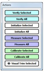
This panel is used to perform the major operations in the application. The various buttons will be disabled and enabled depending on the stage of the calibration process.
