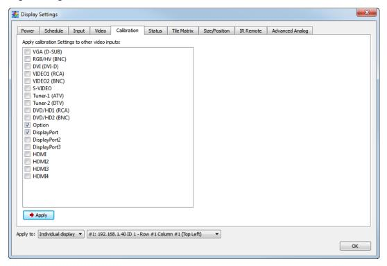
The *Calibration* tab is used to apply the various calibration settings to video inputs other than the input that was selected when the display was calibrated.
