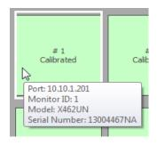
Additional information about a display is shown in a ToolTip by hovering the pointer over a rectangle. This shows the connection information for a display, as well as the Monitor ID, Model Name and Serial Number.
