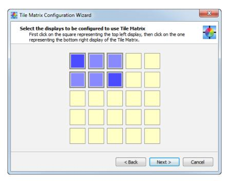
If the video wall is to be divided into multiple groups of displays then the displays in each group can be selected.
