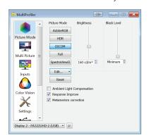
level of correction will give a more uniform screen, but the maximum brightness that can be achieved will be lower. To adjust the uniformity, start MultiProfiler and choose the Settings panel from the icons on the left. Using the slider, change the Digital Uniformity Correction to the desired level.
