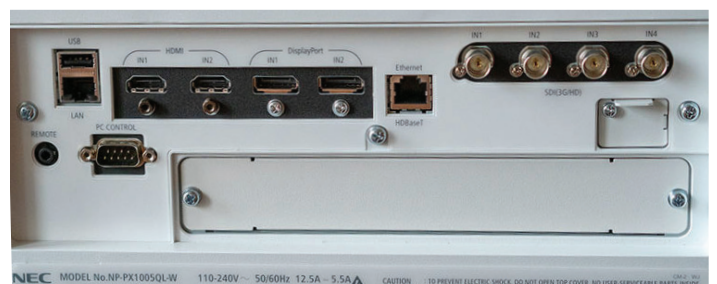
NEC MODEL No. NP-PX1005QL-W 110-240V 50/60Hz 12.5A 5.5A CAUTION TO PREVENT ELECTRIC SHOCK, DO NOT OPEN TOP COVER. NO USER-SERVICEABLE PARTS INSIDE.
