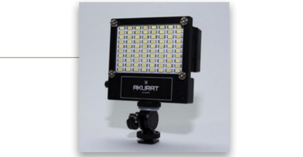
The barndoors and diffuser option are meant to control the light. Using magnets on the front bezel, they're extremely easy to attach and detach from the unit. The diffuser glass sits loosely between the unit and the barndoors and does double duty as a protection for the LEDs. You don't lose f-stops when using it.
