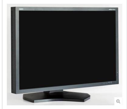
It uses the same AH-IPS panel part from LG Display but adds a 14-bit color lookup table along with a factory calibration, accurate sRGB and Adobe RGB presets and an even more rugged chassis. It looks built to withstand years of daily use not just as a large display but as a professional's tool.
