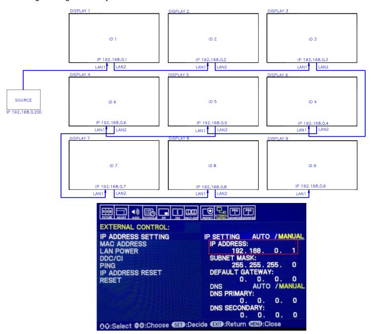
9. Ensure that video source is connected to the DisplayPort In interface of display 1. Make sure that all displays are on the DisplayPort input. Note that the DisplayPort out on each display can be used to output the DVI, HDMI, OPTION or DisplayPort signals that are coming in to that specific display, however, when the next step is completed the display will
