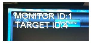
7. Use the TileMatrix feature to setup the 2x2 Video Wall. The Tilematrix feature of the NEC Display allows for one image to be expanded and displayed over a 2x2 Video Wall Setup.\* This is accessed through the OSD (On-Screen Display) Controls under the "MULTI-DSP" main menu icon. Under the TileMatrix sub-menu, enable the feature and set the necessary
