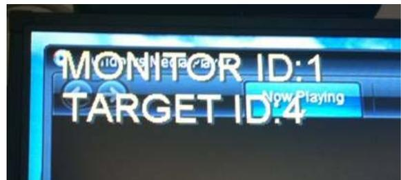
7. Use the TileMatrix feature to setup the 3x3 Video Wall. The Tilematrix feature of the NEC Display allows for one image to be expanded and displayed over a 2x3 Video Wall Setup.\* This is accessed through the OSD (On-Screen Display) Controls under the "MULTI-DSP"
