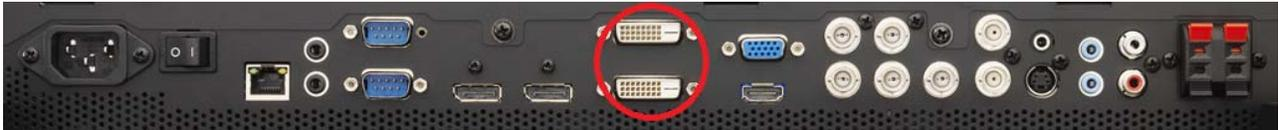
The ideal cabling set up is shown below to match the ideal monitor ID configuration. However, DVI daisy chaining can be done different ways and still yield the same results. Note that the connections for each X463UN monitor are on the bottom of each display, not the side as shown in the image below. It may be helpful to start wiring before mounting.
