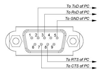
**NOTE:** If so desired, jumper "Request to send" and "Clear to Send" together on both ends of the cable to simplify cable connection. These connections are not required. The only connections required are pins 2 (TxD), 3 (RxD) and 5 (GND).
