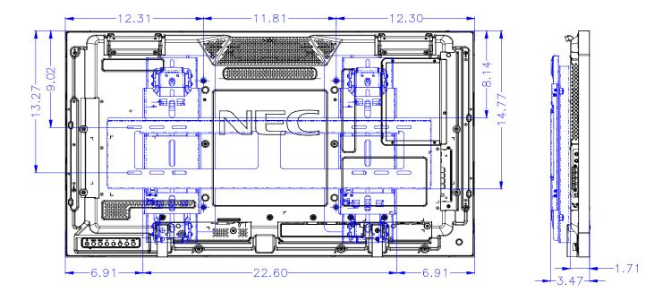
Note: If an OPS option card is installed, offset spacers must be utilized. See WMK-4655S manual.
