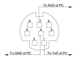
**NOTE 1:** Pins 2, 3, 5, 6 and 8 are used inside the projector..
