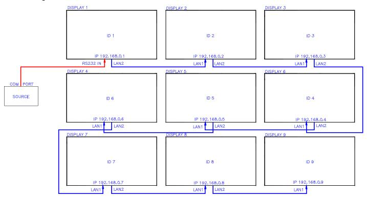
Note that a unique IP address is not necessary to communicate to all displays if display 1 is not connected to a network. The displays will automatically assign themselves IP addresses if no DNS is detected and the IP Setting within the IP Address Setting in the External Control menu is set to AUTO. Note that this is the setting out of the box.
