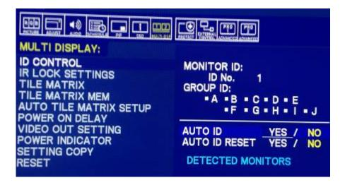
If the control setup is as pictured below, each display does not need a unique IP address assigned to still control each individual monitor.
