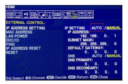
7. If display 1 is connected to a network or LAN is going into display 1, like the picture below, each display will need a unique IP address to ensure that communication can successfully go through the daisy chain from screen to screen.
