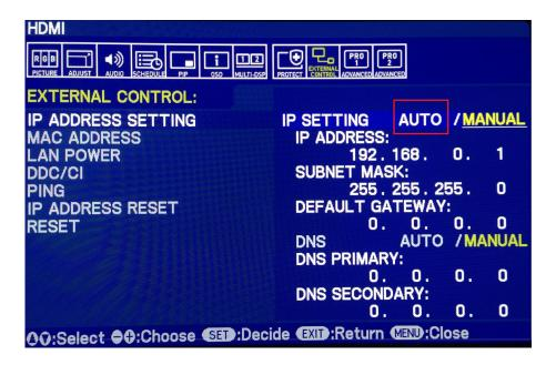
8. If display 1 is connected to a network or LAN is going into display 1, like the picture below, each display will need a unique IP address to ensure that communication can successfully go through the daisy chain from screen to screen.
