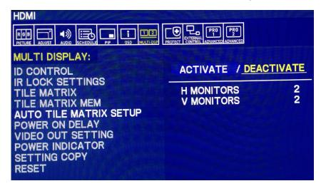
Note that you will need to set the horizontal and vertical monitor dimensions before you activate the Auto Tile Matrix. If done correctly and the LAN is daisy chained as shown on the picture on the previous screen, the displays will automatically adjust so one large picture
