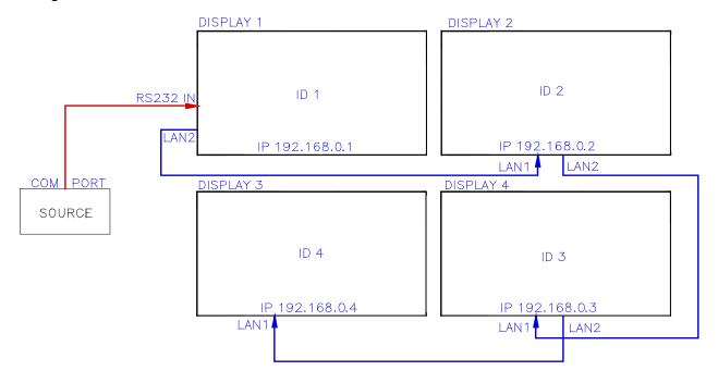
Note that a unique IP address is not necessary to communicate to all displays if display 1 is not connected to a network. The displays will automatically assign themselves IP
