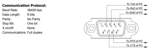
**NOTE 1:** It is recommended to set the projector to "Idle Mode" in the Setup menu for best Power ON response. **NOTE 2:** Pins 2, 3, 5, 6 and 8 are used inside the projector.
