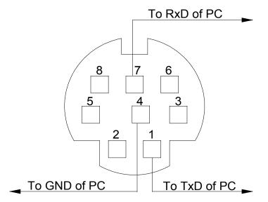
**NOTE 1:** Pins 2, 3, 5, 6 and 8 are used inside the projector. **NOTE 2:** For long cable runs it is recommended to set communication speed within projector menus to 9600 bps. v 3.0
