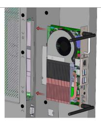
Please make sure that the Slot-in PC (SDM) is always inserted in the righ way.
