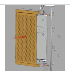
For some public displays the back of the Slot-in PC (SDM) is not covered fully by the display itself. For these displays a back covering plate is included which covers the fan on the Slot-in PC (SDM), making it inaccessible.
