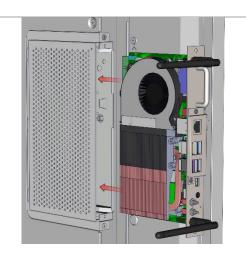
Please make sure that the Slot-in PC (SDM) is always inserted in the right way and pay atention that the Slot-in PC (SDM) slides into the slide rails. Then use the Philipps screws to fix the Slot-in PC (SDM).
