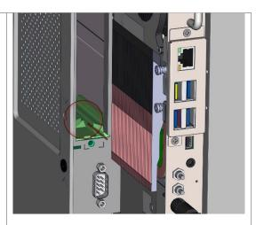
Please pay attention that the Slot-in PC (SDM) slides into the slide rails. Then please use the Philipps screws to fix the Slot-in PC (SDM).
