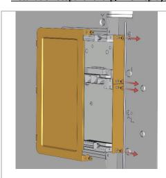
Please remove the slot covering plate by loosening the 4 Philipps screws.
