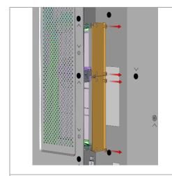
Please remove the slot covering plate by loosening the 4 Philipps screws.
