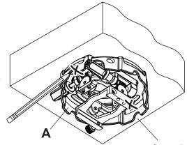
Arrow on top of mount assembly indicates front of mount.
