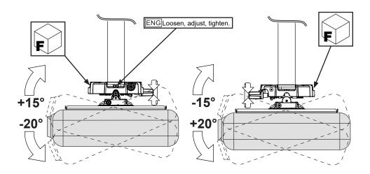
ENG SWIVEL (YAW) 360° (when attached to an extension column), +/- 15° (when flush mounted).
