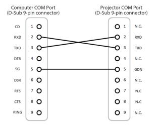
**NOTE 1:** Pins 1, 4, 6, and 9 are not used inside the projector.
