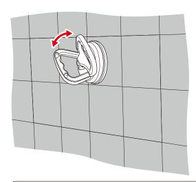
(1) Open the grips of the maintenance tool and push the maintenance tool against the pixel card. Close the grips of the maintenance tool and stick the pixel card.
