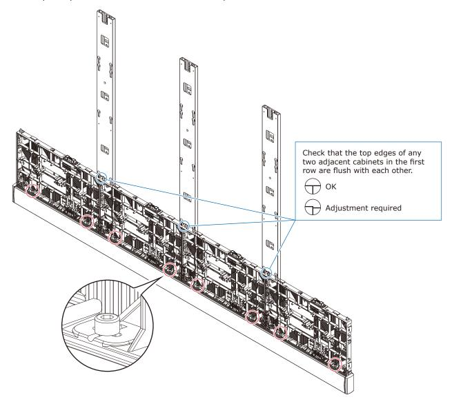
Hook the hanger pins of the cabinets of the second row to the mounting bars. Secure the LED cabinets together using screws for connecting cabinets. Do not tighten the screws completely.
