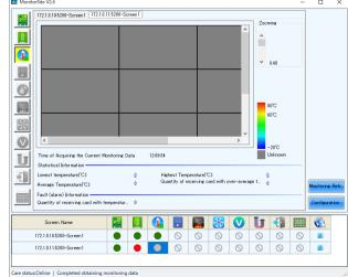
Note: On the monitoring screen, the LED modules configured as "Backup" are displayed in red color (this is not an indication of a fault).
