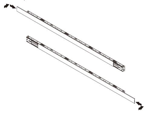
Insert the slot nut into the overframe and align it with the marking line and fix them with screw for overframe screws. Use overframe screws (M4  $\times$  4) for the right side and overframe screws (M4  $\times$  8) for the rest.
