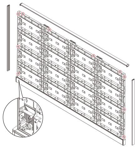
Install the corner parts to the corner frame top and install it on the top of the cabinets.
