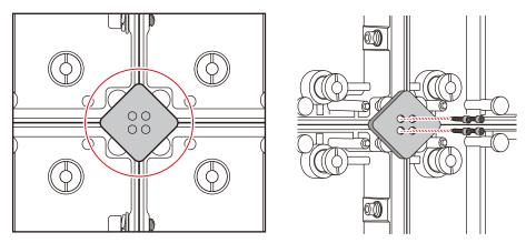
Adjust the position of the cabinet by turning the vertical alignment screw and the back in the center of the vertical alignment screw (cabinet hanger pin) with a flathead screwdriver.
