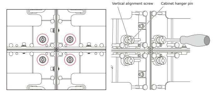
When the cabinets' surfaces are aligned, securely tighten the cabinets of the first row to the power bar, the cabinets of the first row together, as well as the cabinets of the first row with the cabinets of the second row. Remove the Adjustment plates after the screws have been tightened.
