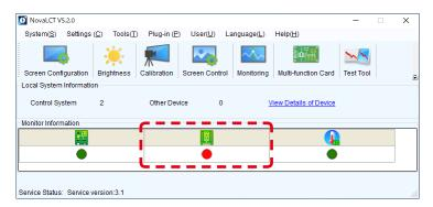
In the case of MCTRL 4K, the display of the LED controllers is as follows. (This example display is for the case of connection using four Ethernet cables.)
