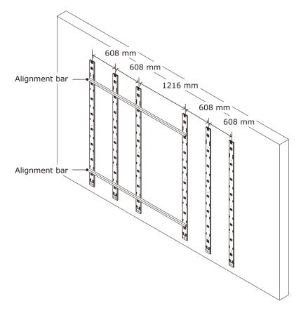
(3) Check the evenness using a spirit level or a laser line level and the alignment bars together. Adjust the positions if required.
