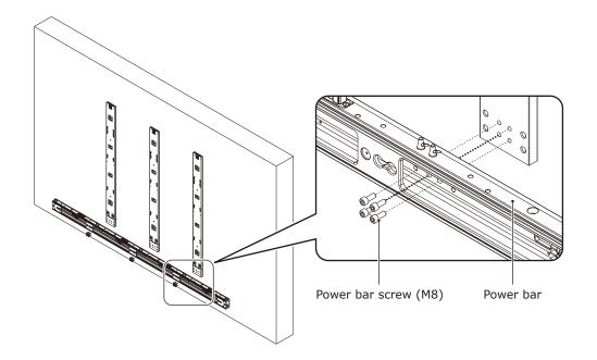
When using the  $8 \times 8$  frame set, use the power bar connecting part to install the power bar.
