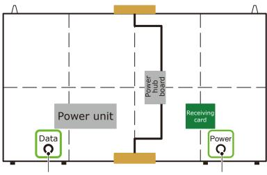
Hole for LAN cable connection
