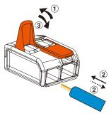
Lever operation is necessary even for connection of a solid core wire.
