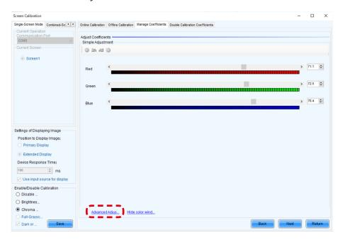
(7) Adjust the "Color adjustment of red, green and blue" parameters, and then adjust the "Color matching of red, green and blue" parameters.
