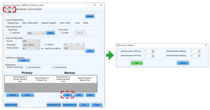
In the Redundancy Settings screen, set the Port to use on the LED controller.
