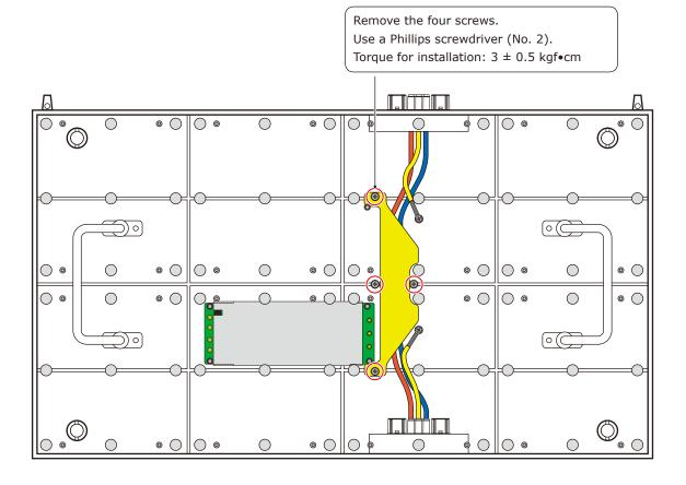
Remove the two screws securing the power unit. Use a Phillips screwdriver (No. 2).
