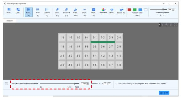
Upward arrow: Increases the brightness (makes the dark lines less noticeable)
