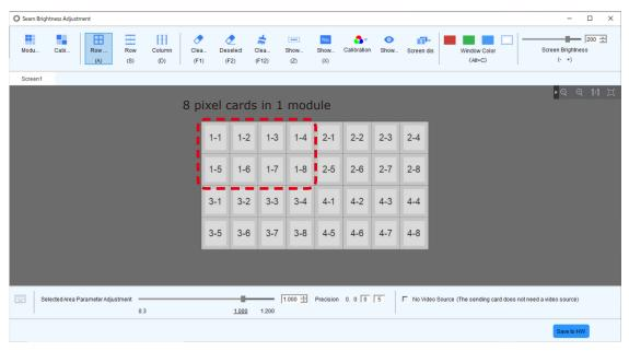
(6) Specify the border between the pixel cards for which you want to perform line calibration by clicking on it or specifying a range. You may also adjust multiple locations at the same time.
