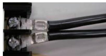
When connecting the cables to the ground terminal block, ensure that parts other than the solderless terminal (such as cable wires and fittings) are not pinched within the terminal fastening area.
