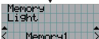
← Select the memory name of the setting to overwrite and press the ENTER button to display the confirmation screen.
