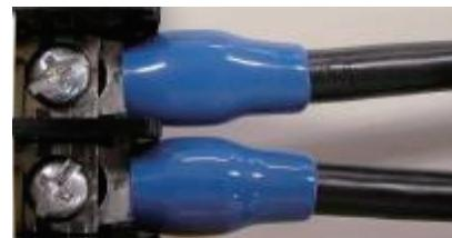
Use sleeves and secure the insulation to ensure that terminals do not touch each other. If the cables are attached to the power supply terminal without using sleeves, there is a risk of the terminals touching each other as shown in the photograph on the right.
