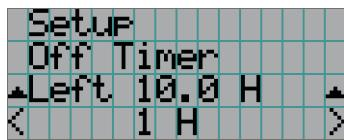
← Displays the remaining time until the power is turned off.
