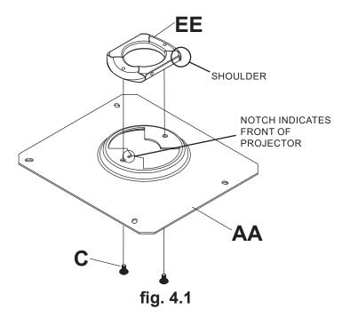
Flip projector upside down and attach adapter plate (AA) using four serrated socket pin screws (BB) and retaining spacers (CC) as shown below. Tighten using 4 mm allen wrench (B).
