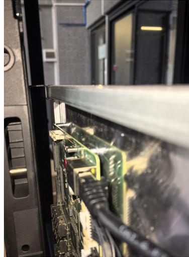
Figure 37 - Install the control box
