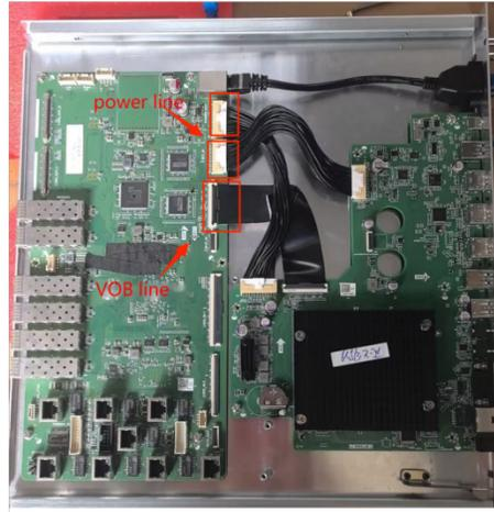
Figure 39 - Send card and SoC board card connected installation physical diagram
