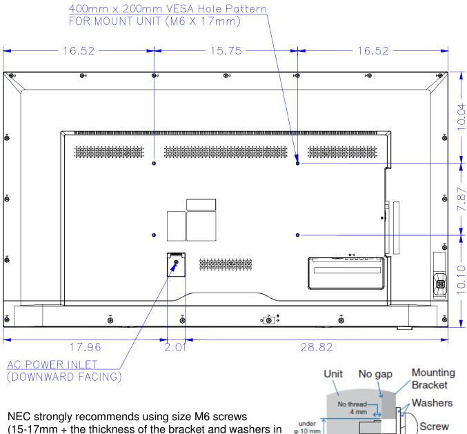
(15-17mm + the thickness of the bracket and washers in length). If using screws longer than 15-17mm, please check the depth of the hole.
