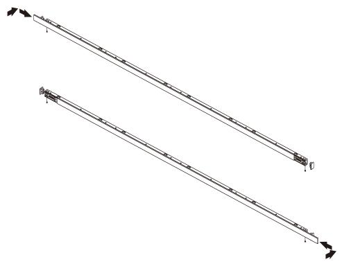
Insert the slot nuts inside the over frame into the holes of the screw for connecting cabinets and fix them with M3 screws.
