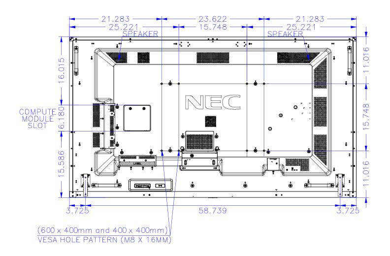
NEC strongly recommends using size M8 screws (15-17mm + the thickness of the bracket and washers in length). If using screws longer than 15-17mm, please check the depth of the hole.
