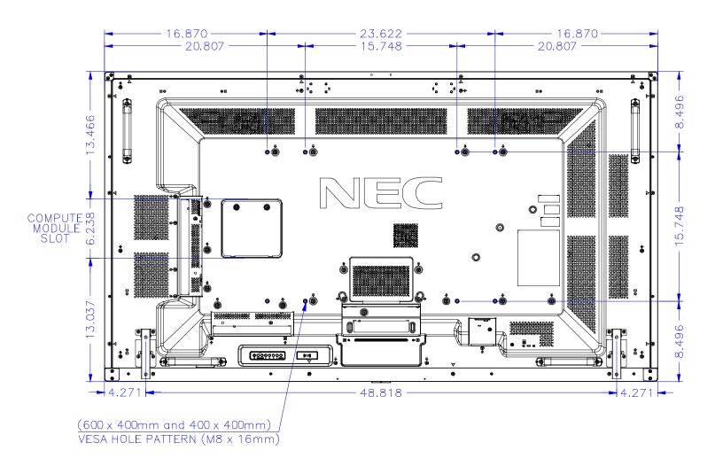
NEC strongly recommends using size M8 screws (15-17mm + the thickness of the bracket and washers in length). If using screws longer than 15-17mm, please check the depth of the hole.
