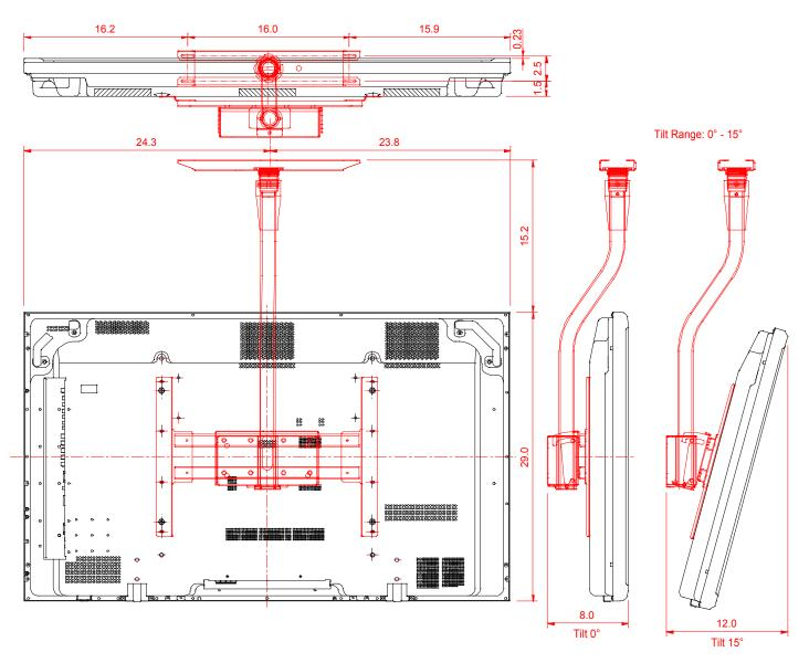
**Note:** The mount holes are 1.14" higher on the 50XM3 than on the 50MP2(PX-50XM2) due to a higher center of gravity. (mount pattern is the same)
