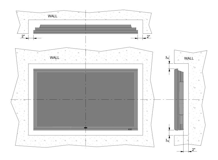
**NOTE:** The ventilation space should not be covered or closed off at the front of the opening. If for some reason the opening needs to be covered, other means of ventilation will need to be incorporated into the design. Contact NEC for design review and recommendations.
