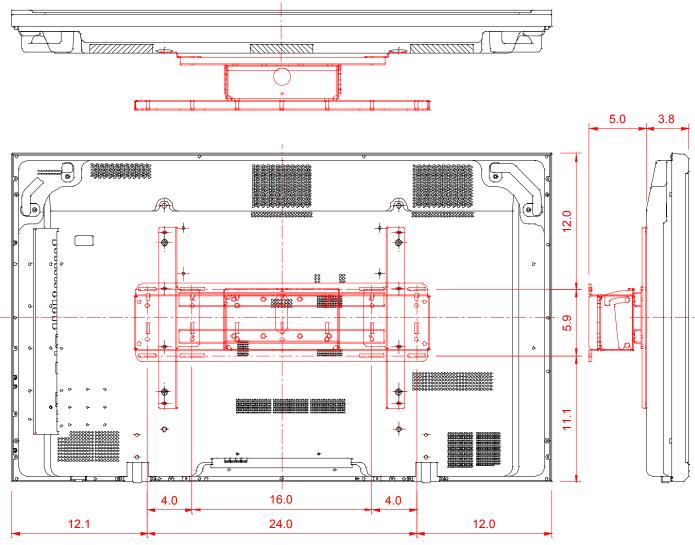
**Note:** The mount holes are 1.14" higher on the 50XM3 than on the 50MP2(PX-50XM2) due to a higher center of gravity. (mount pattern is the same)
