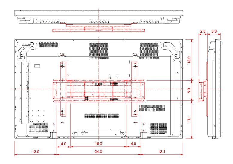
**Note:** The mount holes are 1.14" higher on the 50XM3 than on the 50MP2(PX-50XM2) due to a higher center of gravity. (mount pattern is the same)
