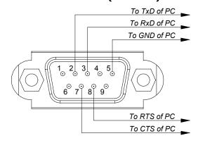
NOTE: Jumper "Request to send" and "Clear to Send" together on both ends of the cable to simplify cable connection.
