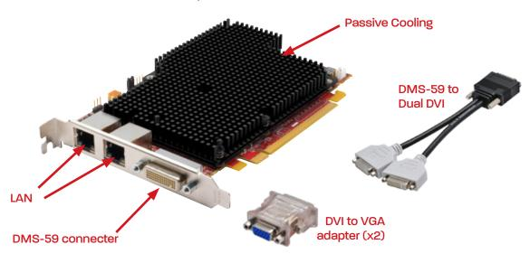
*Mean Time Between Failure (MTBF)*. Passive cooling on AMD FirePro<sup>™</sup> graphics cards uses heat displacement to cool the GPU, which means no fan, fewer moving parts and high MTBF.
