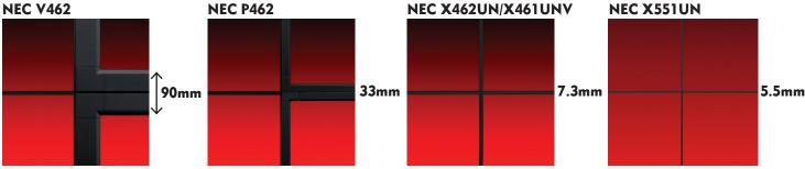
The X551UN's ultra-narrow bezel allows for a screen-to-screen distance between two neighboring displays of only 5.5mm, a more than 1500% improvement over the standard bezel width from NEC's 90mm V Series and close to 500% compared to its previously revolutionary 33mm P Series displays.
