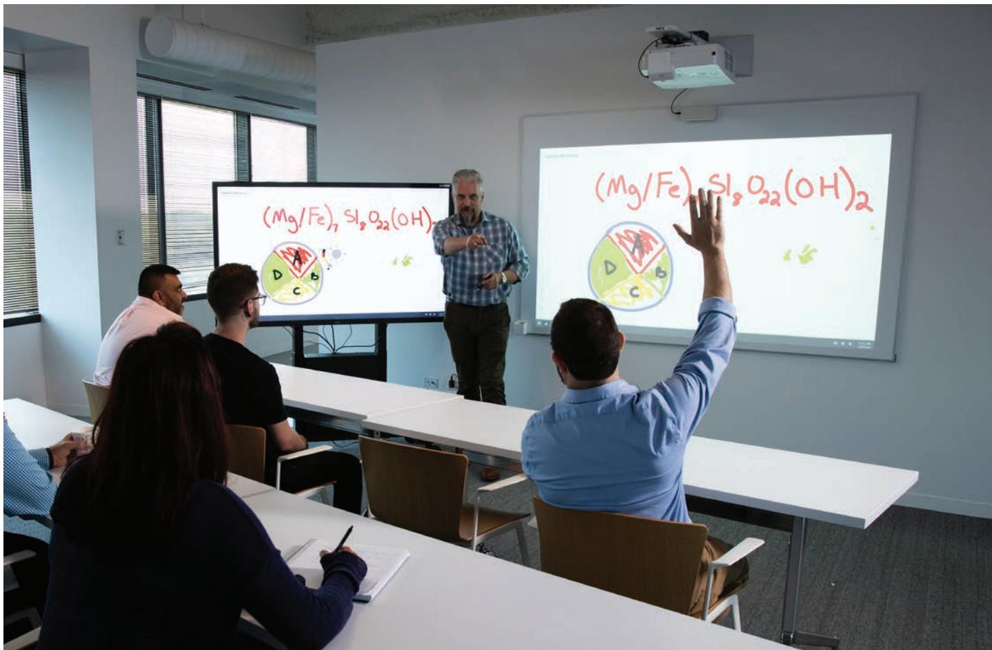
The projector displays a 90-inch diagonal image on a low-glare whiteboard surface. Incorporated interactive modules allow for pen-based and touch control of an attached computer directly from the projection surface. In addition, an interactive large-format display is featured on a rolling stand to complement the collaborative experience. A desktop display and attached computer is used as an individual workstation that can be wirelessly connected with Mosaic software.
